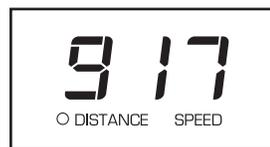
The center display will show the selected unit of measurement. To change the unit of measurement, press the Enter button or the Speed increase button.
