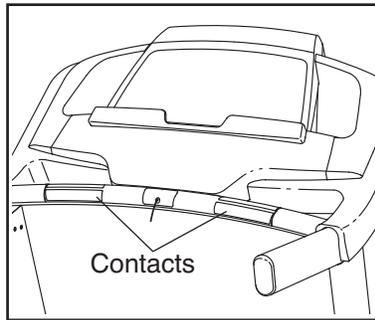
To measure your heart rate, **stand on the foot rails** and hold the pulse bar with your palms on the metal contacts; **avoid moving your hands**. When your pulse is detected, several dashes will appear and then your heart rate will be shown. **For the most accurate heart rate reading, continue to hold the contacts for about 15 seconds.**
