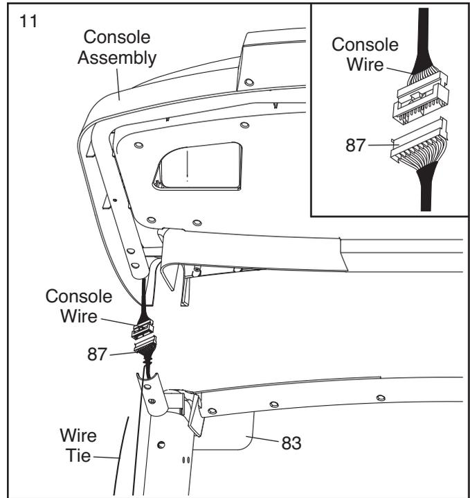
12. Set the console assembly on the Left Handrail (82) and the Right Handrail (83). **Be careful not to pinch any wires.** Insert the excess Upright Wire (not shown) into the Right Handrail.
