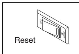
**IMPORTANT:** The console features a display demo mode, designed to be used if the treadmill is displayed in a store. If the displays light as soon as you plug in the power cord and press the power switch into the reset position, the demo mode is turned on. To turn off the demo mode, hold down the Stop button for a few seconds. If the displays remain lit, see THE INFORMATION MODE on page 22 to turn off the demo mode.
