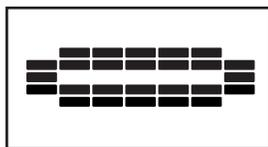
**The Incline/Calories display**—This display will show the approximate number of calories you have burned. The display will also show the incline of the treadmill for a few seconds each time the incline of the treadmill changes.
